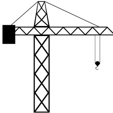
The crane can rotate by  $360^\circ$  and has a height of 20 m between floor and crane boom. The crane boom is 15 m long. The trolley stops 2 m away from the rotation axis. The hook can be lowered until reaching the ground.
